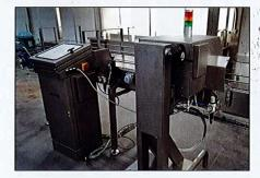
ControlLevel XR is energy-efficient as it requires a lower cooling temperature. The product's most critical components are designed to last longer due to the updated detector and softwarecontrolled x-ray generator that ensures the machine only operates at maximum power when the containers are in the measuring bridge.
