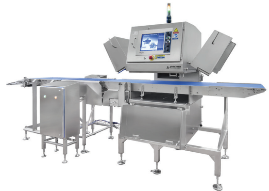
Figure 3: The Eagle RMI3/B unit has been engineered and built with American NAMI and European EHEDG standards with IP69 ingress protection. The machine's louvers open fully making washdown operations—even under intense, high pressure and temperatures—simple, fast and can be completed by one person in a few minutes.
